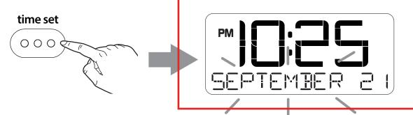
Press the - or + button to set the date (hold for rapid adjust).
