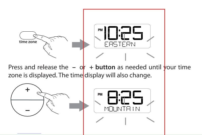
Press and release the **time zone button** to confirm time zone setting.
