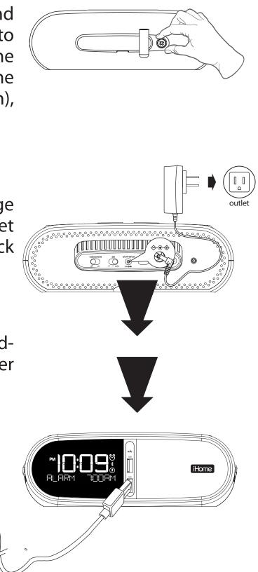
Connect the universal voltage AC adapter to the wall outlet and the DC jack on the back panel of the unit.
