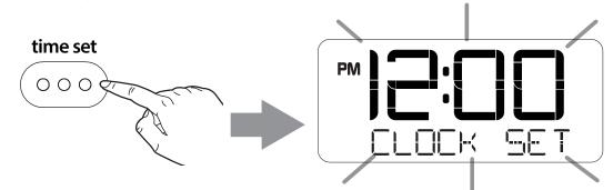
Press the - or + **button** to adjust time (hold for rapid adjust). Make sure to set the correct AM or PM time.
