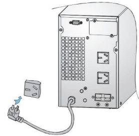
Figure 3-1 Connection Method of Input
