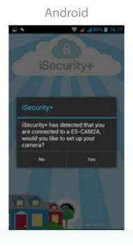
Once the connection has been made (after around 30 seconds), launch iSecurity+. iSecurity+ detects automatically your camera. Select 'Yes' to start the setup of your camera.
