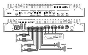
$System\ 2-P650\ used\ in\ 6-channel\ mode.\ Channels\ 1/2\ are\ high-passed\ for\ front\ speakers.\ Channels\ 3/4\ are\ high-passed\ for\ midrange\ speakers,\ and\ channels\ 5/6\ are\ low-passed\ for\ subwoofers.$
