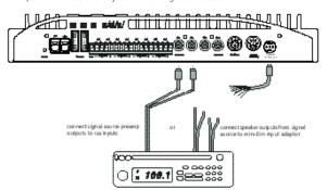
High-level MiniDin input connections:
