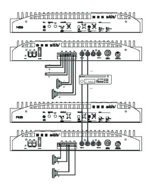
System 1 – P650 used in 6-channel mode. Channels 1/2 are high-passed for front speakers. Channels 3/4 are high-passed for rear speakers. Channels 5/6 are low-passed for subwoofers. Although shown with 4-channels of input, the source unit can be either 2- or 4-channel.
