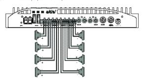
speaker connections for bridged configurations
