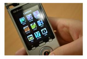
Press the **menu** button to access the menu Select 'Camera' using the cursor and OK buttons
