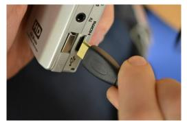
To connect to an **HDMI socket**, use the cable provided and plug the smaller end into the socket (1) above.
