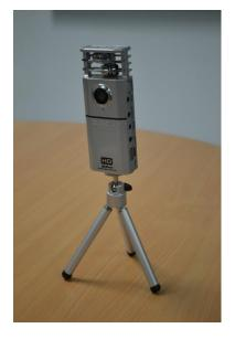
Line the tripod head with the hole in the bottom of the camera.
