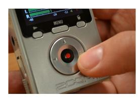
Whilst recording you can **zoom** in and out by pressing the cursor button left or right.
