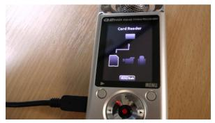
Insert a **USB cable** into the **USB Port** on the side of the device.
