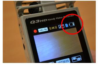
If low, you can replace the batteries by sliding the battery cover
