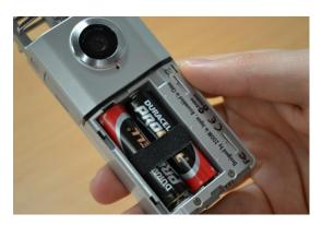
Remove the existing batteries, and replace with new ones, ensuring they are inserted the correct way round
