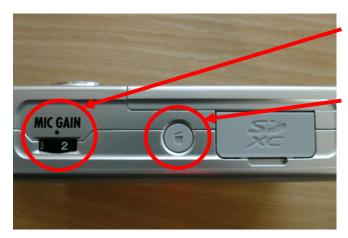
**MIC GAIN** controls how much noise the mic picks up. The higher the number, the louder your recording will be.
