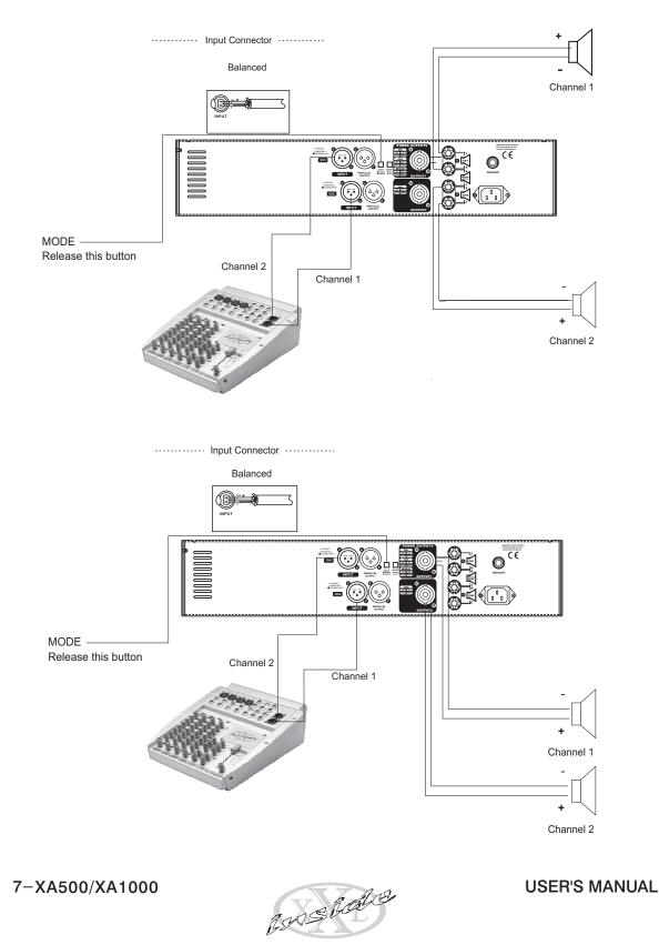
You can also operate the paralleled mode via outside wiring, so, the signal input from channel 1 or 2 will be output from both channel 1 and 2 simultaneously. The volume of channel 1 or channel 2 can be controlled separately.
