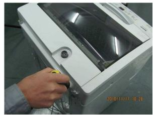
First use cross-style screwdriver to demount the two screws fixed on the back plate. Then use slotted screwdriver to warp the back plate assembly, and sway the back plate assembly gently, then the back plate assembly can be removed.
