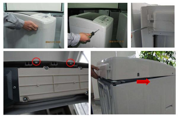
First open the zygomorphous screw cap on the top plate, then demount the two screws by cross-style screwdriver. Second demount the two screws behind the top plate, slant the top plate, demount the seven screws on the control circuit board complete, pull out the jack, then the control circuit board complete can be removed.
