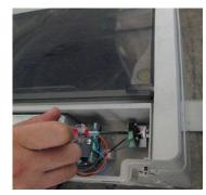
Use cross-style screwdriver to demount the two screws fixed on the safety device switch, pull out the jack, draw the safety device switch out from the slot.
