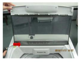
Open the washer lid, move the hinge shaft on the asher lid with slotted screwdriver, then remove the washer lid.
