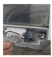
First remove the back plate, then use cross-style screwdriver to demount the three screws fixed on the pour inlet assembly, pull out the jack, draw the pour inlet assembly from the step surface.
