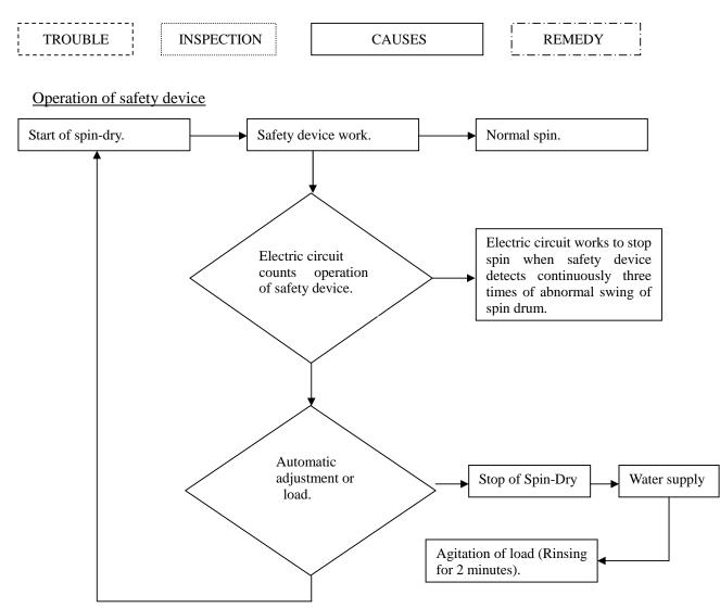
When the safety device works by abnormal swing of spin drum, machine works automatically to stop Spin-Dry cycle and operates water supply valve to pour water into the Wash/Spin Tub and then starts washing cycle for replacing washing clothes evenly.
