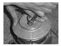
First of all, the outer tub drum assembly must be removed. Demount the two screw assembly on the motor complete, then the motor complete is demounted. At the same time, the motor pulley is removed for it is
