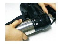
2.Pull downwards until it comes off.Sometimes the impellers will jam the motion when the steel column is being pulled off. Shake the column slightly from side to side to detach the steel column. The pump cap can be removed prior to detaching the steel column.
