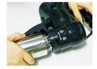
3. Detaching the Pump Cap: Turn the pump cap clockwise.
