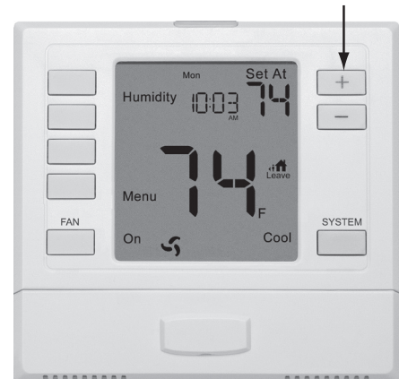
TARGET HUMIDITY SETPOINT KEYS
