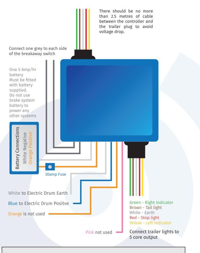
Wiring diagram above applies to SE Brake Controller with electric drums only
