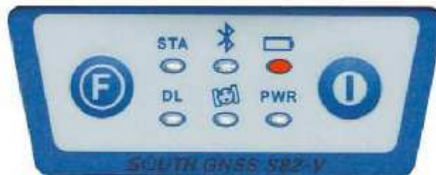
Fig. 2.11 - S82V battery power LED
