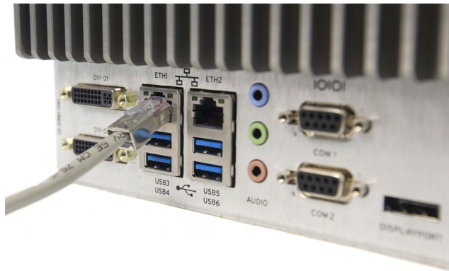
Figure 8 Ethernet Network Connection
