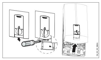
► Open the appliance by pulling the flap downwards, undo the screw and lift up the appliance cover.
