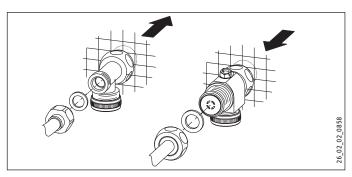
Fit the pipes with flat gaskets onto the twin connectors.
