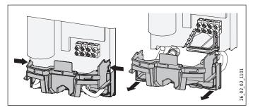
Remove the back panel by pressing the two locking hooks and pulling the lower section of the back panel forwards.
