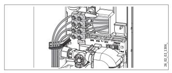
Lay the control wires below the wire guide.
