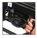
6. Pull the pull starter cord lightly, until it tenses, then pull briskly.
