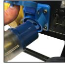
2. Unplug any appliances/ tools that are plugged into any outlets on the generator.
