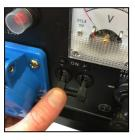
2. Turn the circuit breaker to the 'off' position.
