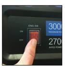
3. Switch the generator to the 'OFF' position.
