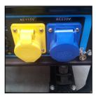
1. Disconnect all equipment cables from the 230 V and 115 V outlets.
