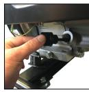
1. Remove the oil reservoir filter cap.
