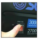
5. Switch the engine switch to the 'on' position.
