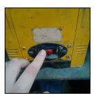
1. Switch OFF any appliances/tools that are plugged into any outlets on the generator.
