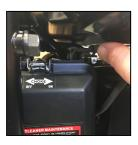
7. Once generator engine starts, move choke lever over to the right.
