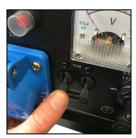
2. Turn the circuit breaker to the 'off' position.
