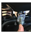
3. Turn the fuel tap downwards, this means the fuel supply is 'on'.
