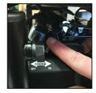
4. Turn the fuel tap so it is pointing 'LEFT' into the off position.
