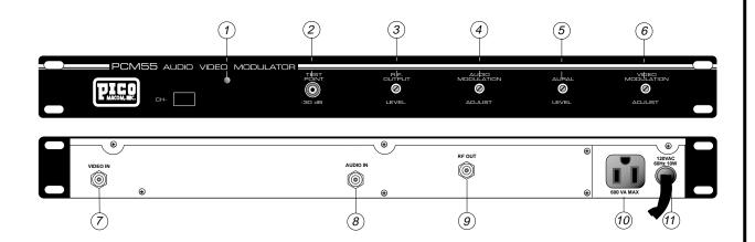
The PCM55 modulator is a crystal controlled modulator. The modulator's operating frequency is determined by the frequency of a high accuracy temperature compensated crystal. The video is applied through a front panel controlled potentiometer to an integrated circuit. The amount of video applied to the IC determines the depth of modulation. A surge
