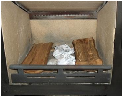
1. Put 2 small logs on a bed of ash spaced about 6-7cm apart. Place some scrunched up newspaper/paper with 1-2 firelighters in between .
