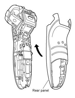
5. When putting the housing A and the housing B together, make sure if the waterproof seal must be fitted properly and no foreign substance sticking around.
