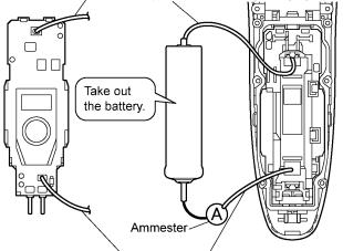
Lead wire of (+) side for checking charging current
