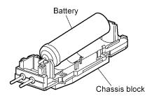
6. Unsolder the lead wires from the module.
