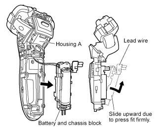
4. Make sure that the lead wires set in position to avoid abnormal noise. Install (+) terminal of battery into the terminal plate at the bottom cover side and firmly set the battery sliding the direction of arrow. Attach (-) terminal of battery.
