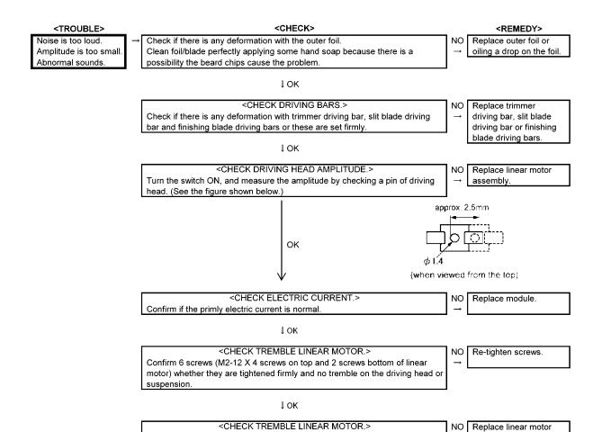
Hold linear motor assembly and check if the tremble sounds stops.
