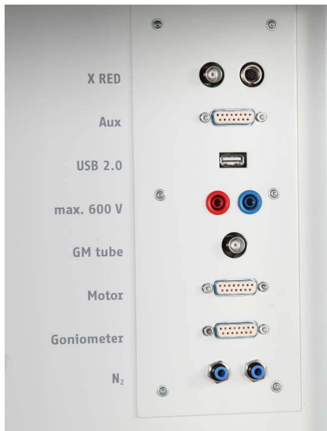
Fig. 7: Socket panel inside the experiment chamber
