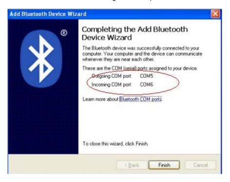
**Step8:** Now if you want to test if the printer is OK to print, you could use a com tool, and send printed data to **Outgoing COM port**(here, it is **COM5**).
