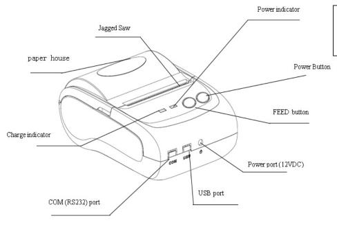
Model: OCPP-M05 Size: 102X78X46 mm Weight: 134g(with Battery))
