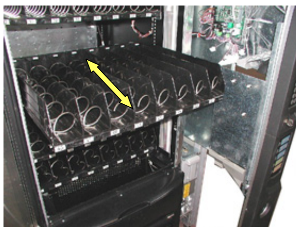
Tray with configuration of 8 single sectors - View while being removed
