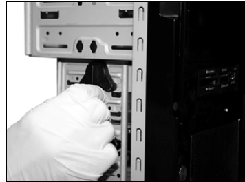
Screwless for 3.5" external device.
