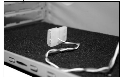
4-pin 120mm front fan molex connector
