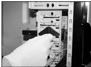
Screwless for 3.5" internal device ( ie Hard drives )
