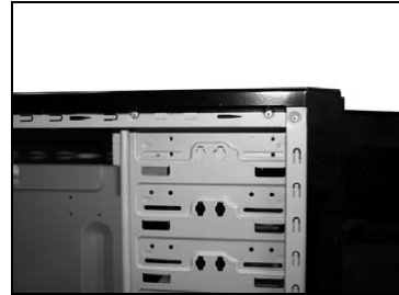
Matching the holes to the 5.25" device.
