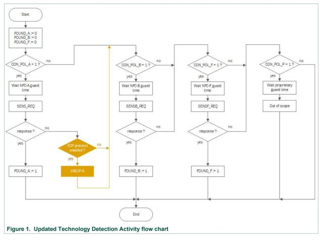
As described in above flow chart, the Apple Enhanced Contactless Polling is only handled when Type A polling is activated. When enabled, the VASUP-A command is inserted approximately 780µs after the Type A initial request (SENS\_REQ).
