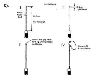
3). Attach the throttle cable assembly to the TMX Carburetor.
