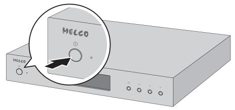
**3** The display panel will change as the sequence below. When the home screen is displayed, the boot process is finished. It will take about 20 seconds to complete.
