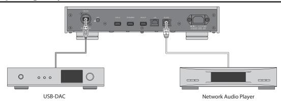
To use a USB-DAC as a player, connect the USB-DAC using the USB cable to the USB-DAC port. After turning the USB-DAC on, you may be able to play music files by changing the input to USB. You can use other ports than the USB-DAC port, but only one device will be detected if 2 or more USB-DAC devices are connected at the same time.
