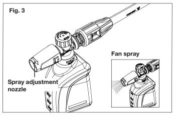
3. With the nozzle tip adjusted to a low-pressure fan spray, apply detergent from the bottom to the top of the dry surface to be cleaned. Applying detergent in this manner will dissolve dirt most effectively.
