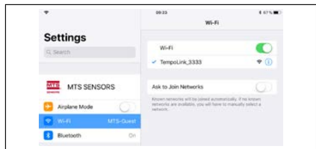
Fig. 5: Choose the network “TempoLink_ xxxx” in the Wi-Fi settings of the Wi-Fi-enabled device
