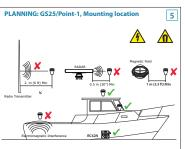
The antenna contains a magnetic heading sensor and should not be mounted within 1 meter (3.3 ft) of any potential magnetic source.
