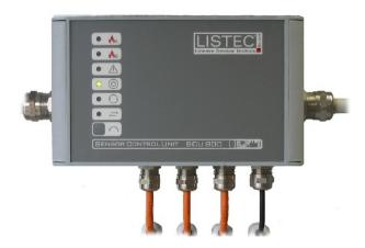
The sensor control unit SCU 800 is the central supervisory element for the d-LIST-system. It provides up to two d-LIST sensor cables with power, performs the cyclic addressing of the connected sensors every 10 seconds, acquires the temperature values measured by each sensor and evaluates the data with reference to various criteria.
