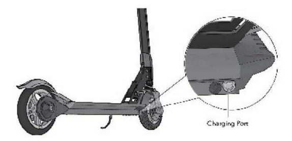
Connect the charger's electric cable to an electrical outlet Open the cover to the charging port in your scooter (note: be sure to keep any liquids away from charging port and cable), and then connect the charging cable to the scooter's charging port under the footboard, on the right side at the front. Always plug the charger into the wall first before the device. The charger o^ers a charging status on the top of the charger: **Charging Light Red** Battery is charging.
