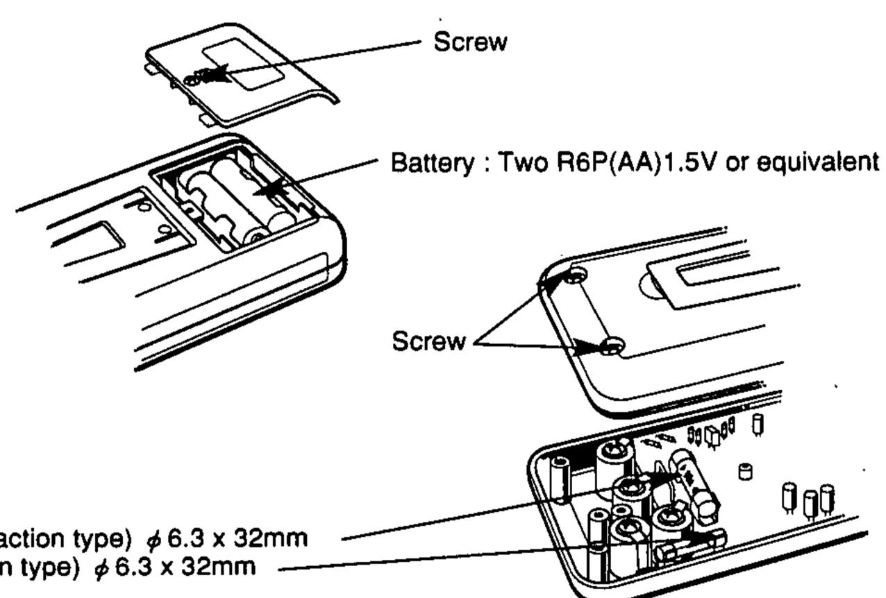
Fuse: F 600V/10A (Fast action type)  $\phi$  6.3 x 32mm F 600V/800mA (Fast action type)  $\phi$  6.3 x 32mm  $\rightarrow$
