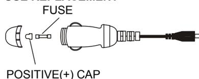
NOTE: Don't throw out the positive(+) cap when replace the fuse.
