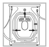
3. Remove the 3 protective screws and the rubber washer with the respective spacer, situated on the rear of the appliance (see figure).
