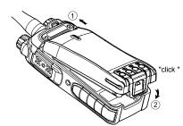
Note: To remove the battery, turn off the radio first, and then slide the battery latch upwards to unlock the battery.
