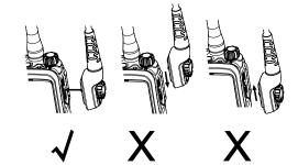
Step 3 Tighten the screw on the plug.
