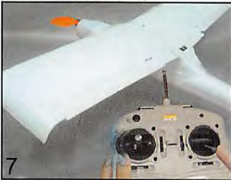
7 Aileron stick move to right. The right side aileron on the airplane will move up, and left aileron move down.
