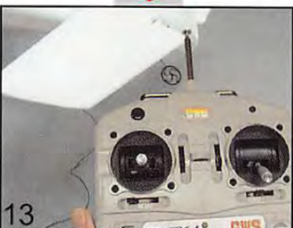
13 When the stick is in neutral, the elevator should return to neutral.
