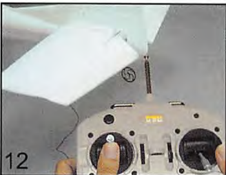
10 Moving the stick up should move the elevator down.
