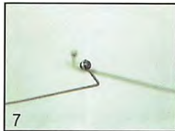
• Push the rubber grommet into a coil of the aileron linkage wire.
