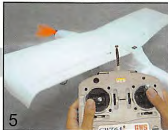
5 Push up the throttle stick slowly and watch the reaction of the motor. The motor should run from low to full throttle as you adjust the stick upward.
