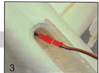
3 Connect power wires and turn on the receiver.
