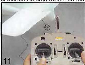
11 Moving the stick down should move the elevator up.
