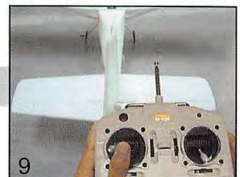
9 Moving the stick to the left should move the rudder to the left.
