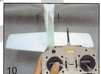
12 Moving the stick to the right should move the rudder to the right.
