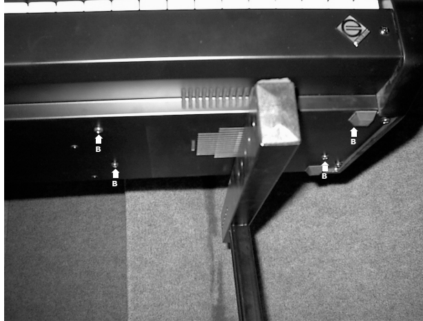
Fig.2 To remove the keyboard unscrew the 10 fixing screws (B) underneath it.
