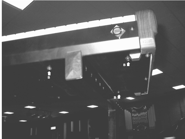
Fig.2 To remove the keyboard unscrew the 11 fixing screws (B) underneath it.
