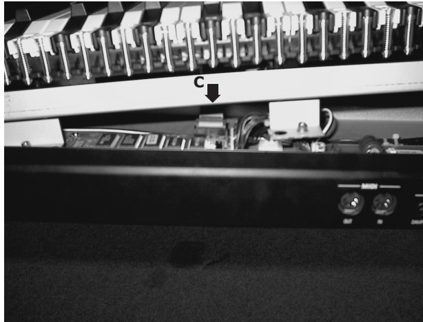
Fig.4 BE CAREFUL: disconnect the keyboard cable (C) without forcing it when you remove the keyboard, to connect the keyboard out of the chassis is needed a longest cable (GM ordering code 840532).
