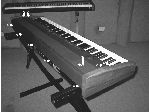
Fig.1 Unscrew the 9 fixing screws (A) and move the front panel towards you and lift it up .
