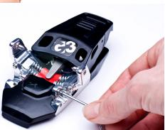
Re-install the Onyx binding toe onto the base plate. Locate the toe in the original position and torque the toe positioning screws to 5.6 N·m (50 in-lbf)
