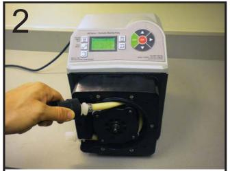
Introduce tubing into pump head while the rotor is rotating. <u>Avoid using fingers to guide the tubing.</u> Stop pump at anytime by pressing **STOP** button. Start pump by pressing **START** button.
