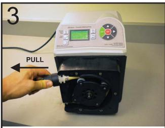
Continue to follow rotation of rotor while directing tube into pump head. At this point, you may need to pull Tube Installation Tool to stretch tubing into position. Let rotor spin a few rotations while pulling Installation tool so fitting can be properly installed.
