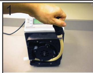
Insert suction fitting into pump head. Remove your fingers from pump head. Start pump by pressing **START** button. Grab hold of Tube Installation Tool and use it to leverage tubing into pump head.
