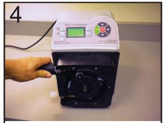
Continue to pull Tube Installation Tool to allow enough room to slide discharge fitting into pump head tongue and groove. Once discharge fitting is secured in pump head, stop pump by pressing STOP button. Replace pump head cover. Pump will ask you if you'd like to reset tube timer. If you choose **yes**, current tube time will display for 5 seconds before resetting to zero. Make note of your displayed tube life. Select Yes again to reset tube life timer.
