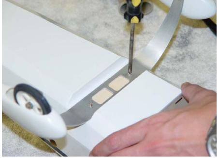
4. Locate the motor box assembly and the 2 laser cut triangular motor box supports. Place the tabs in the motor mount assembly into the firewall and push down so that they lock into place. Install the triangular supports as shown. Wick thin and medium CA into all joints and allow to cure. Locate the 2 clear plastic air scoops and glue them into place as shown.
