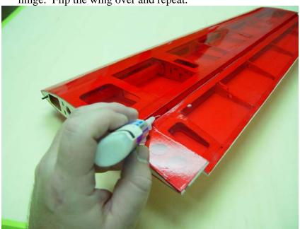
2. Use a #11 hobby blade to remove the covering over the servo bay. Install the aileron servo using the manufacturer supplied mounting screws. Route the servo
