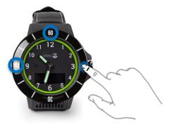
Please note that button functions are enabled or disabled depending on selected DORO SECURE 480 profile. In safety alarm profile the 15, 45 and 60 buttons show the battery level in the display. In Geofence and home beacon profiles none of the buttons are operational.
