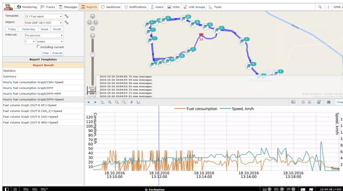
Figure 4 — Example of Analytical Report generated in ORF 4 software, based on the DFM CAN data
