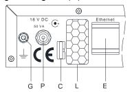
To connect the grounding cable, please take off the upper nut and the first washer of the grounding bolt (**G**). Then connect the grounding cable, which must have a ring tongue terminal matching for the M4 fastening bolt. The washer and the nut have to be tightened again.
