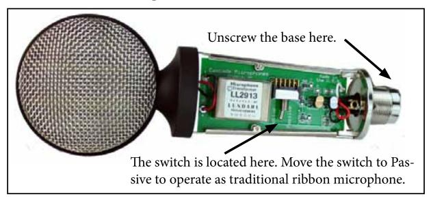
• Reassemble the microphone, keep the phantom power off on the mixer and plug it back in. You will notice now that you will have less gain and the microphone will respond as a normal ribbon microphone. The Lundahl transformer will still be in the circuit.
