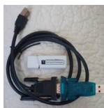
A SERIAL dongle connects to PC's USB port
