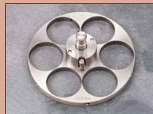
60-2100 Single Force Specimen Holder Plate, With Six 2" (50mm) Cavities. Use distance rings for smaller size specimens.
