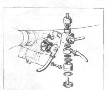
Clean, with compressed air, fuel lines, petcock and carburetor filters, if necessary.
