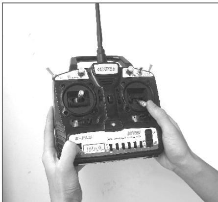
5. Press frequency bind button again to get it rebound. After the indicator light flashes for a few seconds, it turns green, the transmitter get into working mode.
