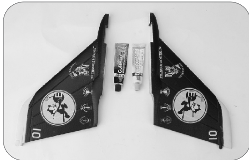
13. Take out the AB glue in the accessory bag and two vertical tails
