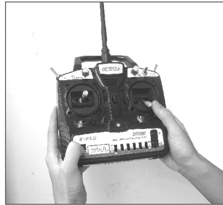
2. Press the frequency bind button, then turn on the transmitter's power.
