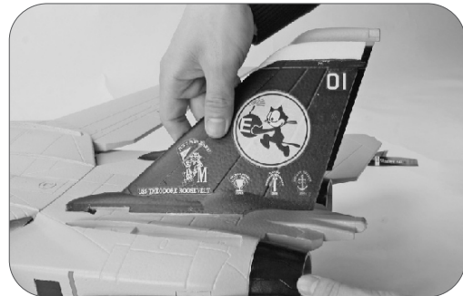
14. Mix the AB glue in 1:1 ratio and spread it on the surface between the vertical wing and the tail of the fuselage, and then paste them together.
