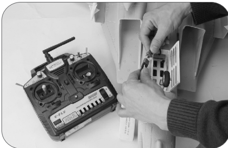
1. Turn on the transmitter, make sure the throttle is on the lowest position, connect the flight battery to the ESC then put it into the battery box.
