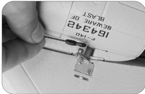
11. Instal the ball buckle of the stabilizer control steel wire to the ball buckle in stabilizer.
