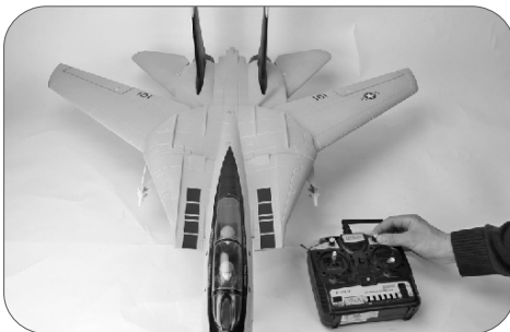
3. Function of the right knob of the transmitter: turn the knob and make the main wing reach the min. sweepback, now by turning the knob you can put the main wing in any position between the max. and min. sweepback.
