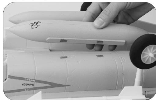
16. Take out two auxiliary tanks and fix them to the proper position below the fuselage by the magnet (It's up to the customer if they want to assemble or not)
