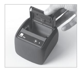
of paper from a new roll and hold the layers tightly wound. Put the new paper roll in the paper compartment, making sure that the outside is turned towards the printer mechanism.
