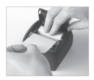
Press on the centre of the lid until it audibly snaps into place. The paper can be torn off at the tear-off edge without the lid opening up and without the paper sliding through the print head.
