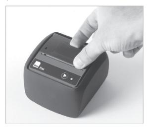
Completely open the lid to expose the paper compartment and remove the empty paper roll.
