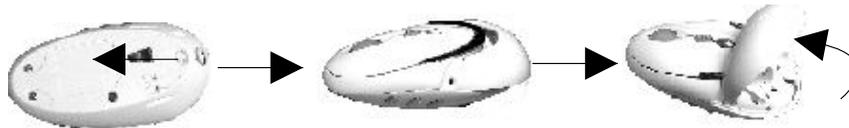
2. Insert 2 AAA rechargeable batteries in correct direction
