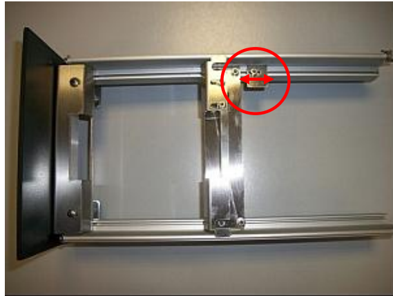
Figure 6 - Drawer Sensor Adjustment
