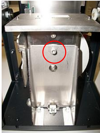
Figure 7 - Front-to-Back Screw Adjustment
