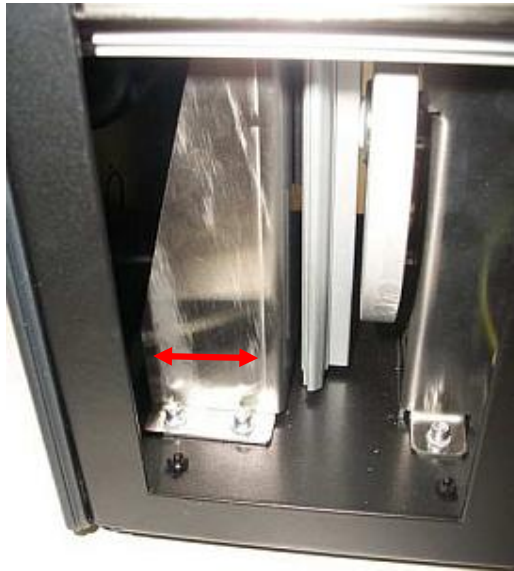
Figure 11 - Adjusting the lift's position
